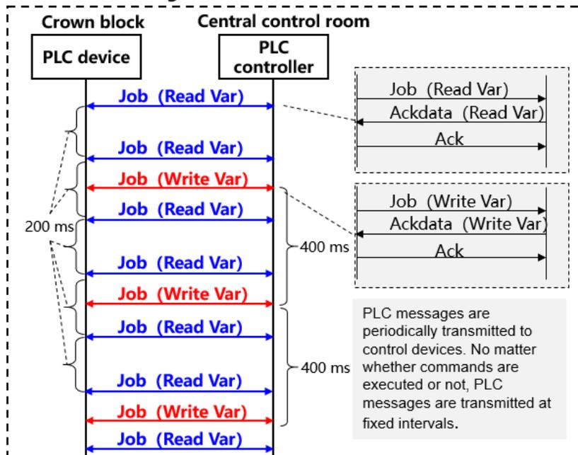
According to the S7Comm protocol, there is no specific protection mechanism for transmission latency. Therefore, even if the network transmission time is long, no alarm is generated (provided that transmission is stable). However, the protocol has a periodic status update mechanism for messages; each time a message is received, the periodic timer is updated.
