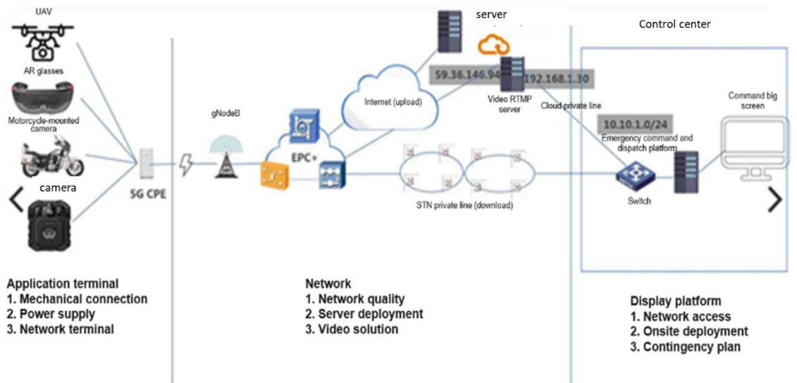
Introduction: 5G network capabilities are leveraged to build a 3D smart video storage and analysis system that uses unmanned aerial vehicles (UAVs), AR glasses, motorcycles.
