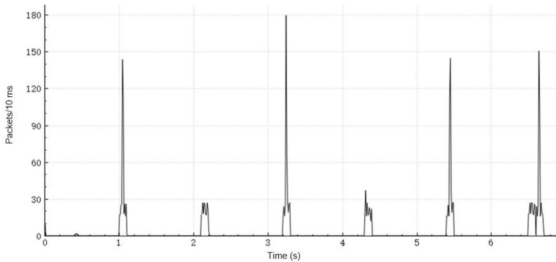
A batch of data is sent per second, and is proactively controlled by the camera video sampling rate. Therefore, the average video upload rate depends on the average video bit rate.
