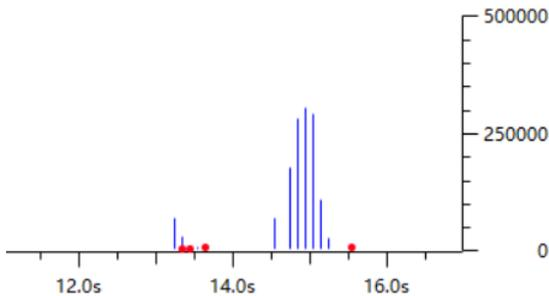
The uplink code stream is shown in red, and downlink code stream in blue. The downlink rate is 2.5 Mbps.
