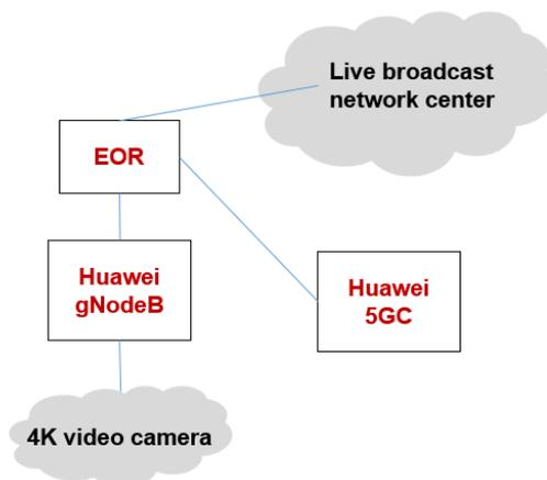
The upload service involves real-time uplink data transmission. The uplink transmission rate is approximately 100 Mbps, which is not necessarily the highest capability of a network. The live broadcast service is transmitted based on the real-time encoding rate of the camera, that is, the average bit rate of 4K videos after real-time encoding is 100 Mbps.
