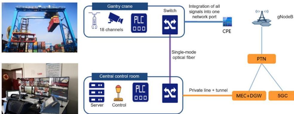
Application scenarios: Remote gantry crane control, automated guided vehicle (AGV) control, and autonomous driving of container trucks
