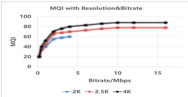
In low-speed industrial automation scenarios (5 km/h), the resolution has a greater impact on user experience than the bitrate. As shown in the preceding figure, the improvement in experience is not obvious when the bitrate is higher than 2 Mbps, 10 Mbps, and 4 Mbps in 2K resolution, 2.5K resolution, and 4K resolution, respectively.
