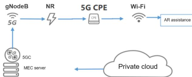
Network requirements: Typical AR glasses are mainly used for 720p video streaming, so 1.5 Mbps downlink rate is required and the latency must be within 20 ms. The 5G + MEC solution is required, as 2K–4K video streams are future demands.
