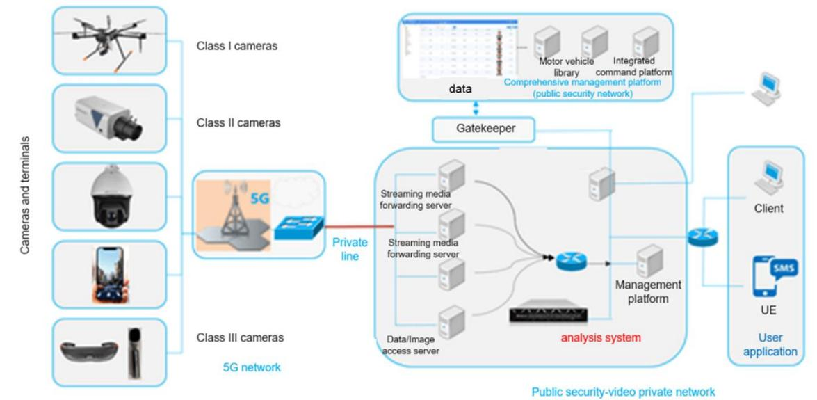
Service introduction: Three types of cameras are connected to the video private network. The analysis server can give object information.
