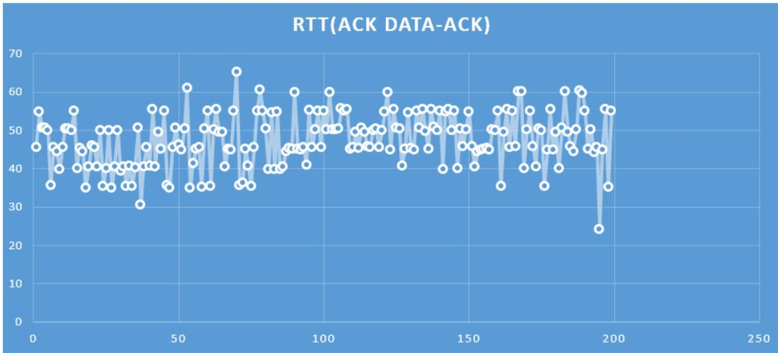
The average latency is 47 ms. Fluctuation is relatively small, ranging from 30 ms to 65 ms; this RTT reflects the network quality from ACK\_DATA to ACK and cannot be covered by Response Delay.
