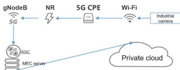
Network requirements: Industrial cameras photograph three images of a module per second. Each image is 300–600 KB and seven to eight cameras upload images simultaneously, so 50–115 Mbps uplink rate is required. After photos are combined and processed on the cloud, the final drawing is less than or equal to 500 MB. Onsite engineers need to download the drawing using a tablet or PC within 3 seconds, so 1.3 Gbps downlink rate is required.
