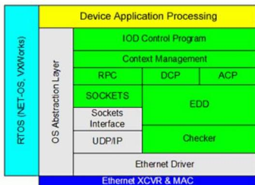
These parts highlighted in green are the protocol stack of PROFINET IO.
