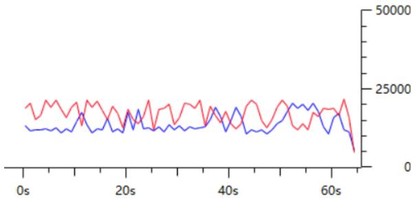
The uplink rate is shown in red, and the downlink rate in blue. The average uplink rate is 18 kbps, and the average downlink rate is about 15 kbps.
