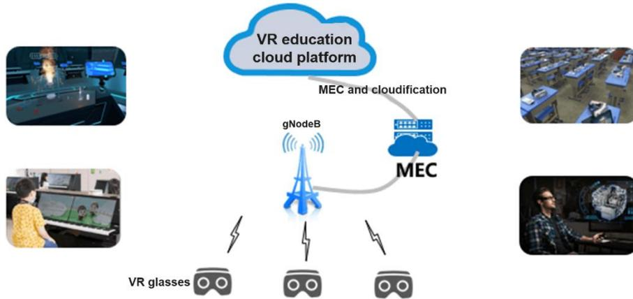
AR/VR teaching contents are uploaded to the cloud. The cloud computing capability is used to implement AR/VR running, rendering, display, and control. The high bandwidth and low latency of 5G are used to transmit the content to VR glasses in real time and construct AR/VR cloud platforms and applications. These include virtual labs, popular science teaching, and 3D interactive classrooms.
