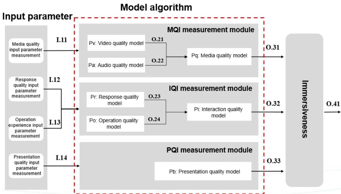
**Figure 7-13** Input and output of AR service quality measurement
