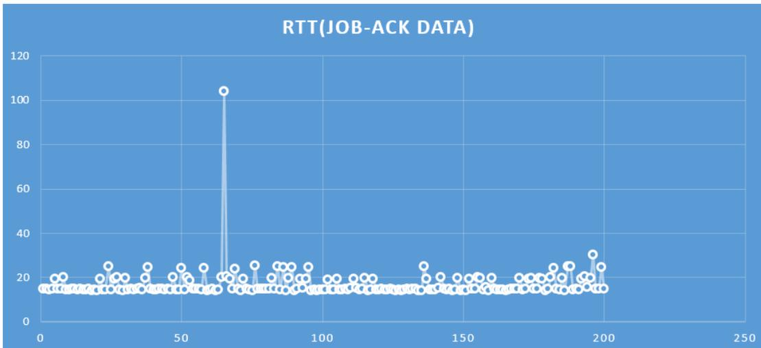
The average RTT is 17 ms. The RTT at one point is large, reaching 104 ms. This value corresponds to the high point of Response Delay in the preceding figure.
