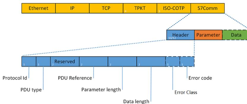
PDU type: indicates the type of PDU. The values are as follows:
