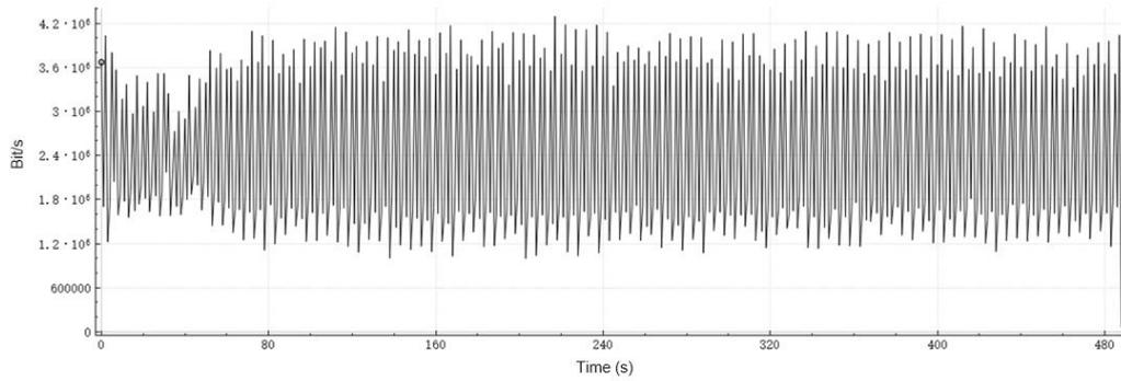
According to the 1-second transmission characteristics, the average rate in a period of time is stable. In particular, the video bit rate is slightly higher than the configured bit rate.
